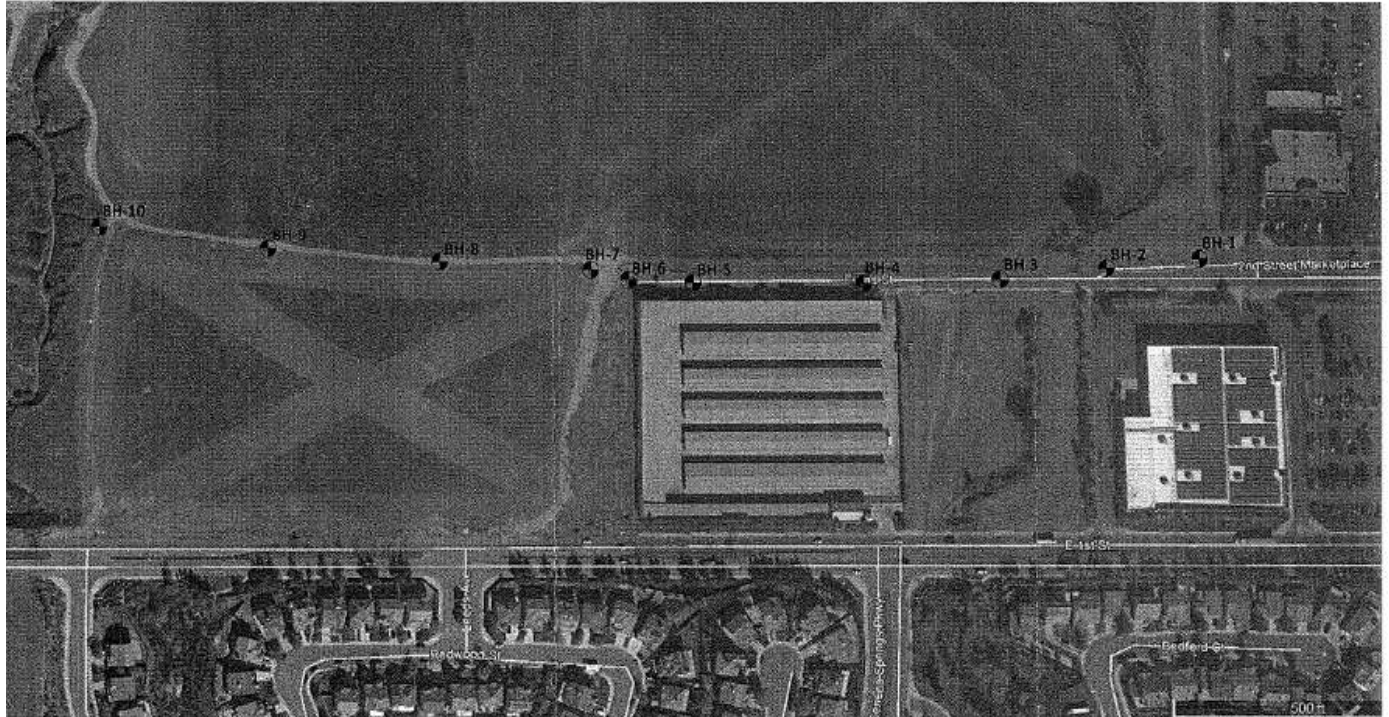
Figure 18. Alignment Showing Borehole Locations for Investigation.
