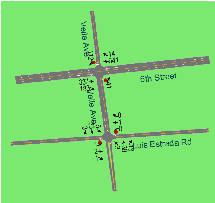
Figure 11 – Existing AM Peak Hour Volumes 6 th St and Veile Ave Veile Ave and Luis Estrada Rd
