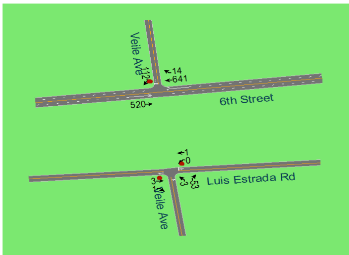
Figure 14 – AM Peak Hour Volumes with the Proposed Veile Ave Roadway Segment Closure Between 6 th St and Luis Estrada Rd
