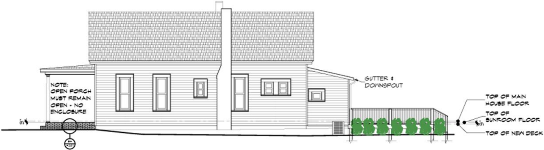
Right side elevation with existing window; rough opening is 62.5"(width) x 39.75" (height)
