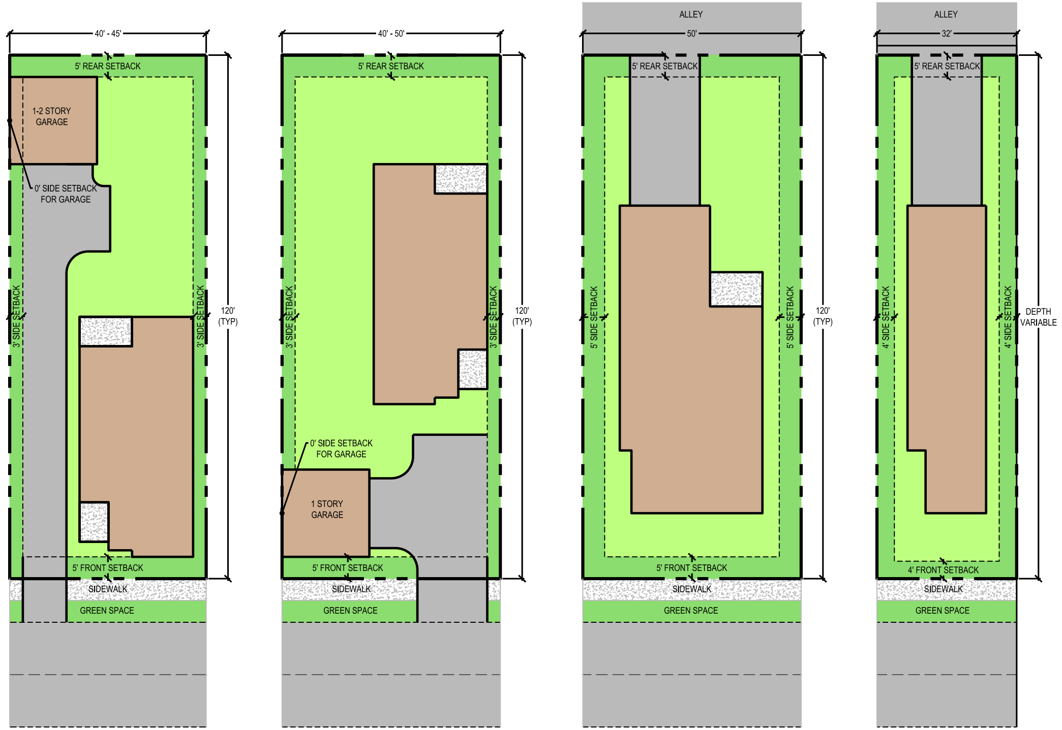
LOT TYPE A BEAU COAST - 40' FRONT LOAD w/ DETACHED GARAGE * OPTIONAL TWO-STORY GARAGE w/ HABITABLE SPACE SHALL HAVE THE SAME SETBACKS AS THE PRIMARY STRUCTURE
