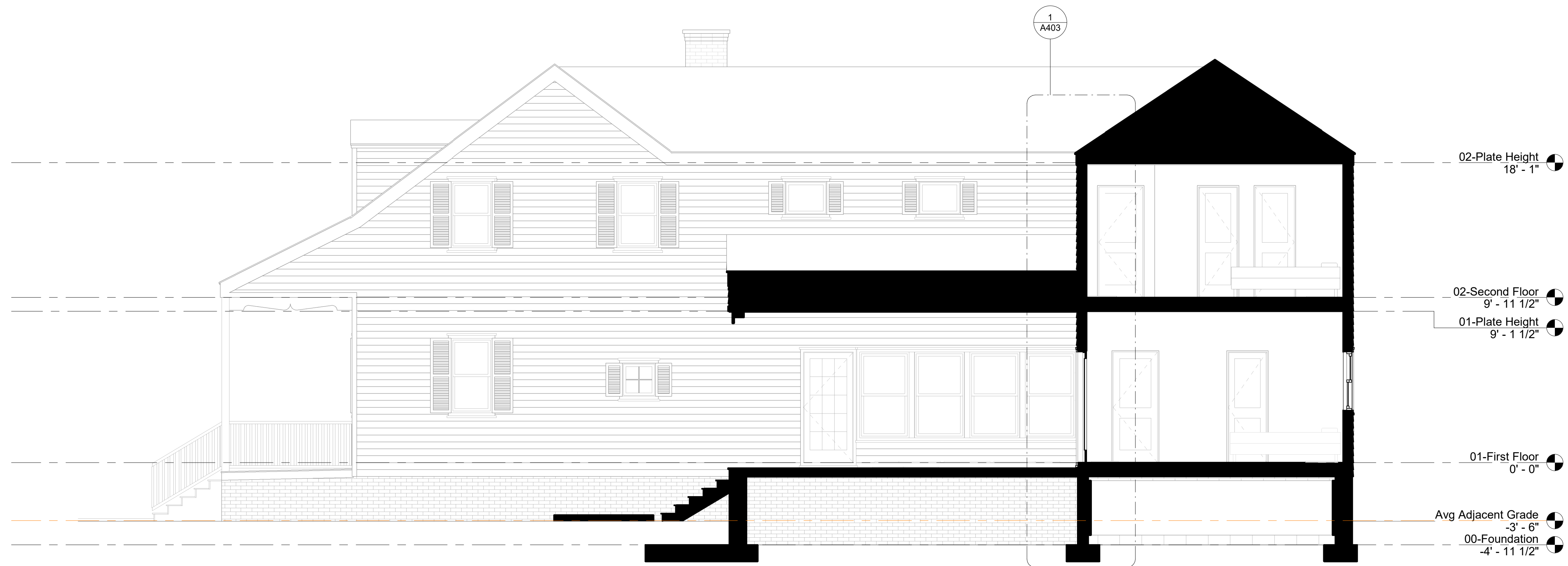
2 Building Section - Side Porch Entry 1/4" = 1'-0"
