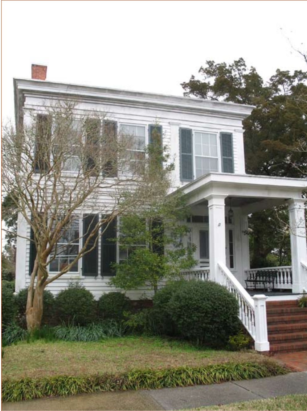
A one-story porch with a flat roof and prominent squared posts or columns is typical of the Greek Revival style in Beaufort.
