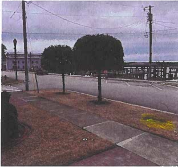
Sidewalk View of Telephone Pole and Live Oaks. Code Requires 35' Distance, not 18', nor 33'. See Utilities 9' to Right of Live Oak 3. Too close.
