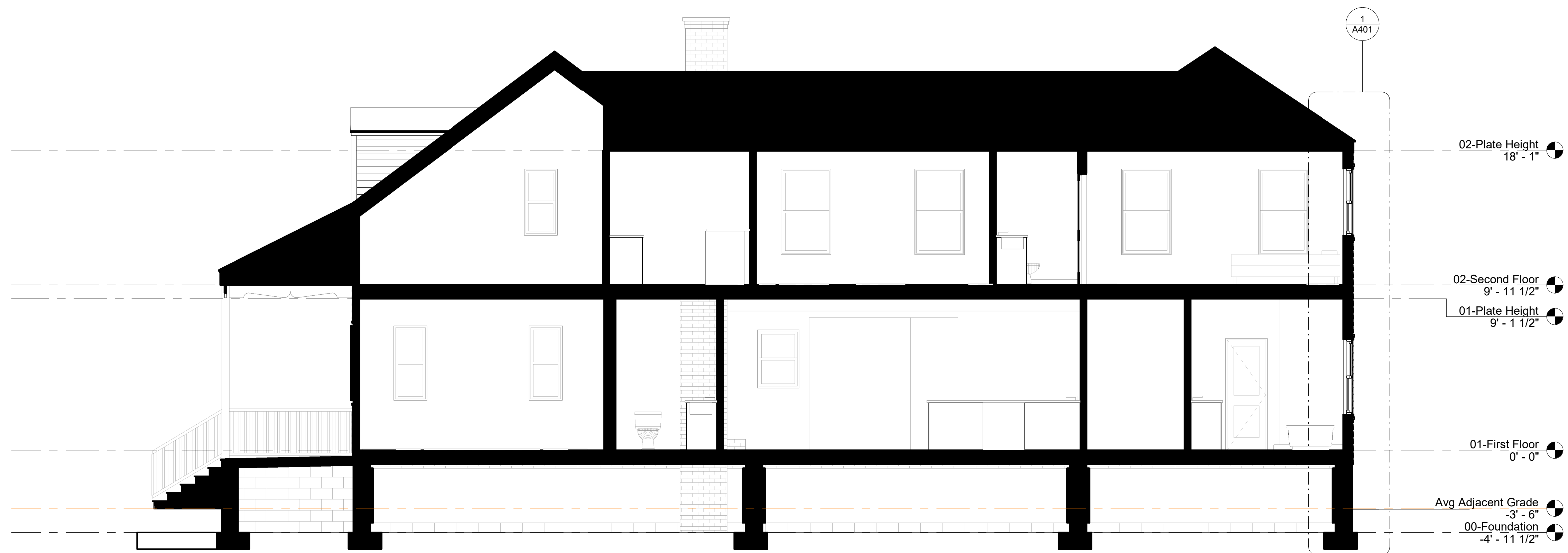
1 Building Section - Rear Addition 1/4" = 1'-0"
