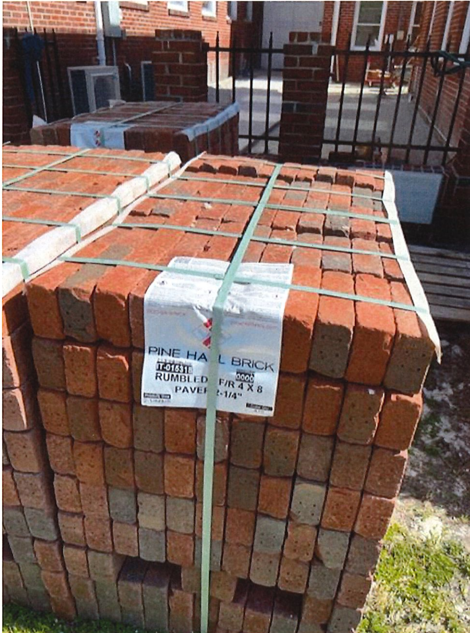
Proposed Pine Hall Rumbled Pavers 4"x8"; Pavers to be used on sidewalk and drive.
