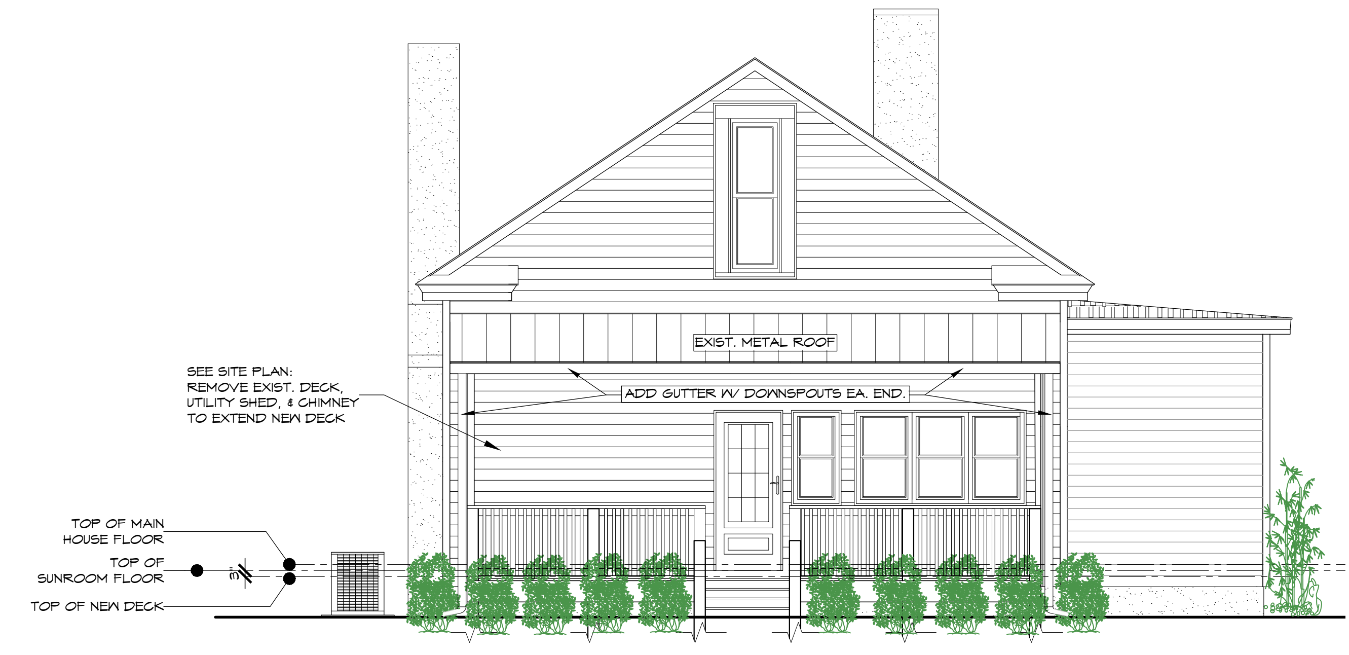
2 PROPOSED REAR ELEVATION W/ NEW DECK A201 SCALE: 1/4"=1'-0"
