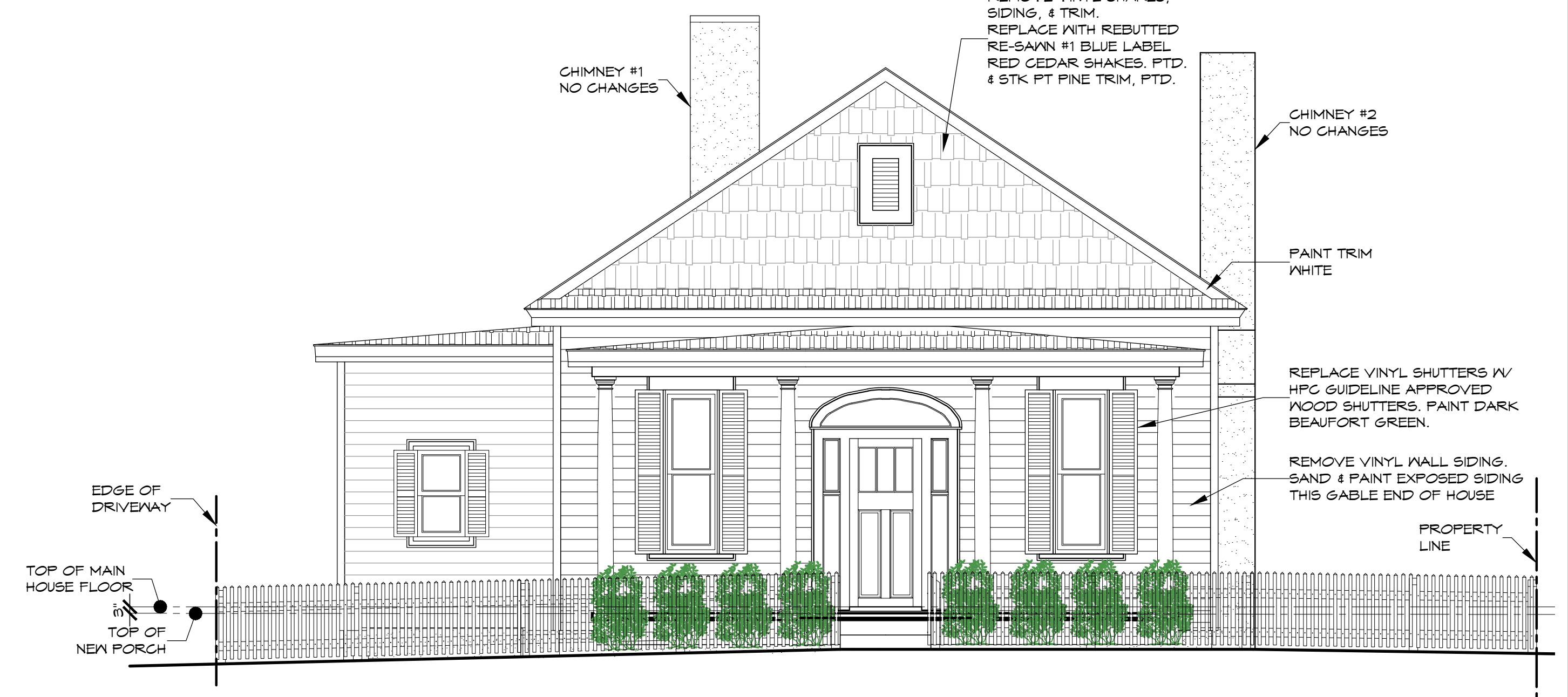
1 PROPOSED NEW FRONT ELEVATION (MOORE STREET) W/ NEW PORCH A201 SCALE: 1/4"=1'-0"
