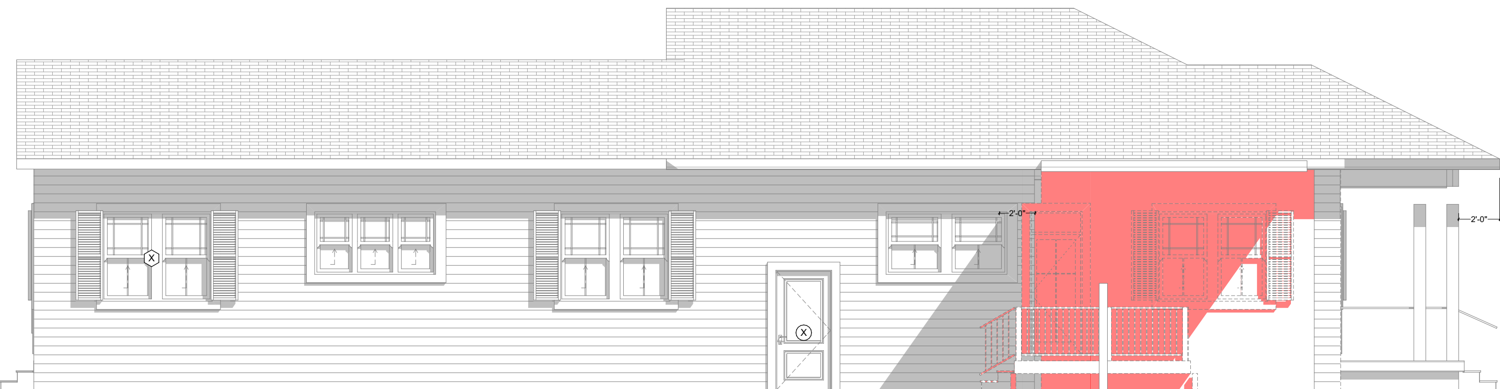
2 West Elevation Demolition Plan SCALE: 3/16" = 1'-0"
