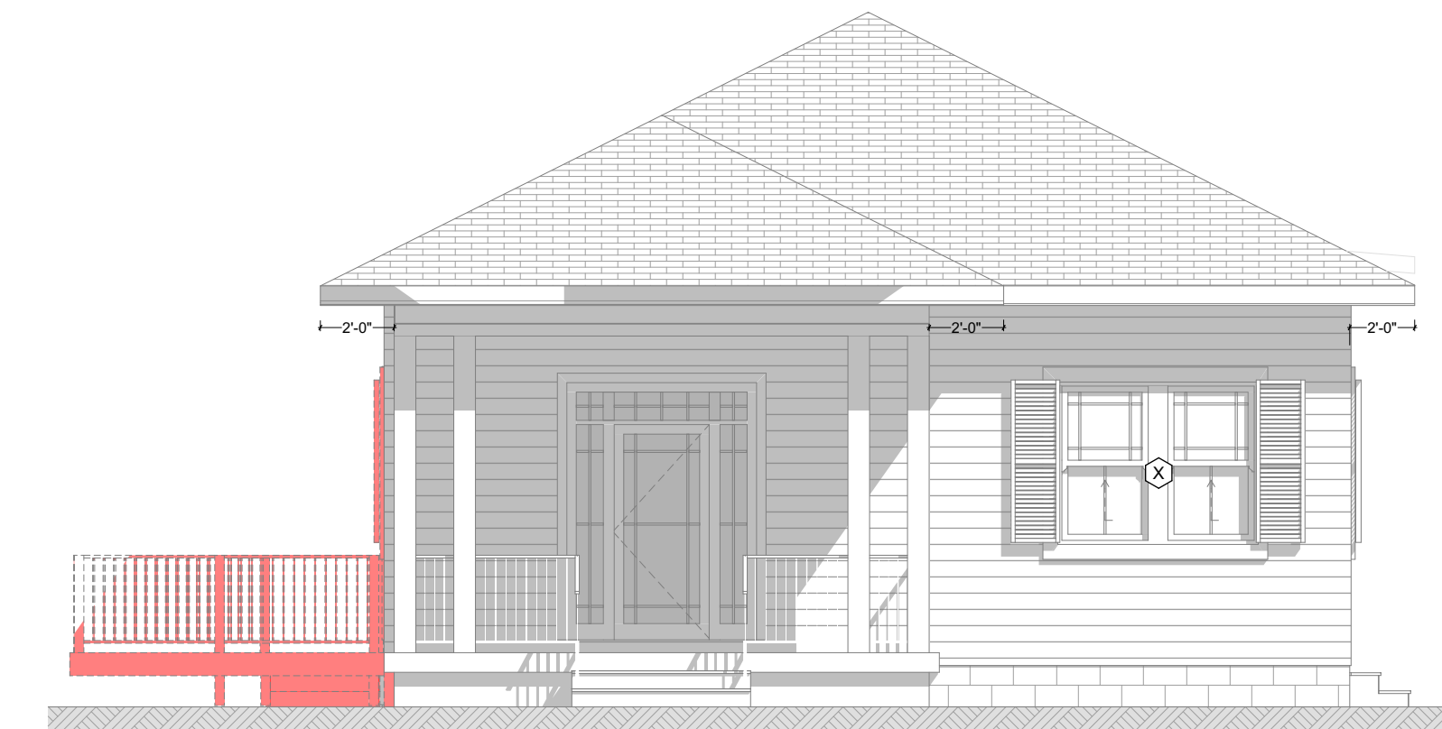
4 North Elevation Demolition Plan SCALE: 3/16" = 1'-0"
