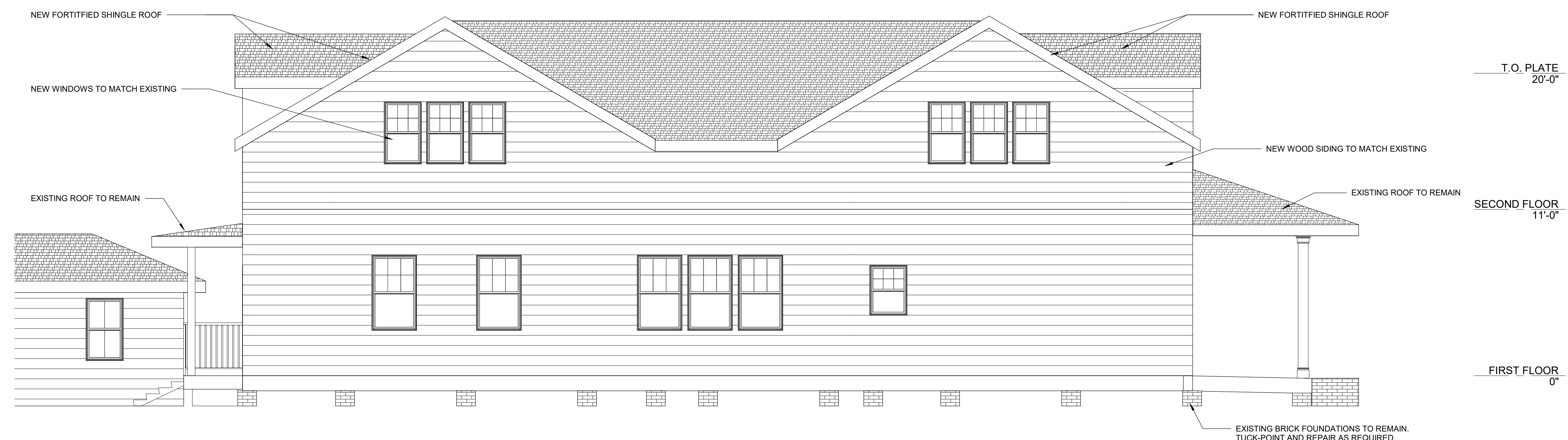
1 A2.1 Left Elevation - Proposed 1/4" = 1'-0"
