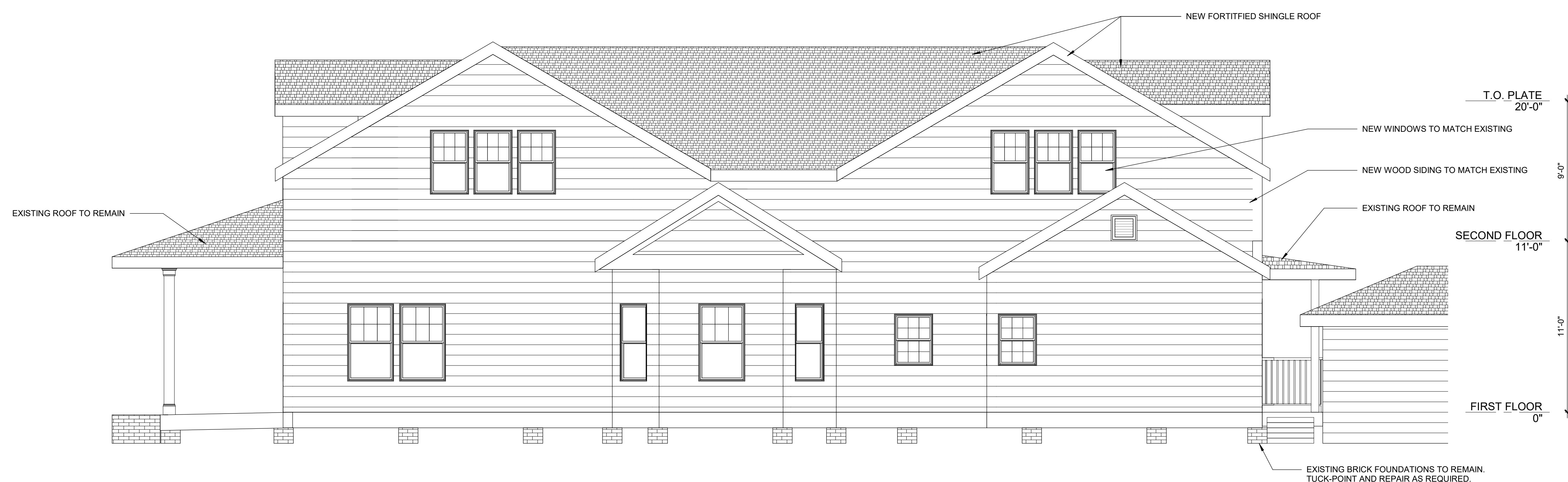
1 Right Elevation - Proposed 1/4" = 1'-0"
