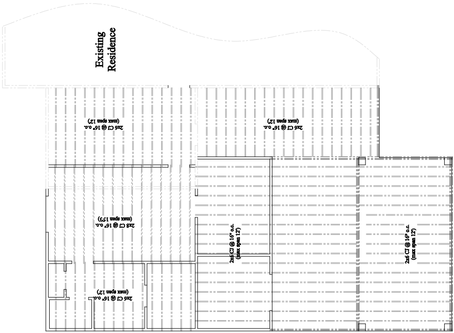
CEILING JOIST PLAN
