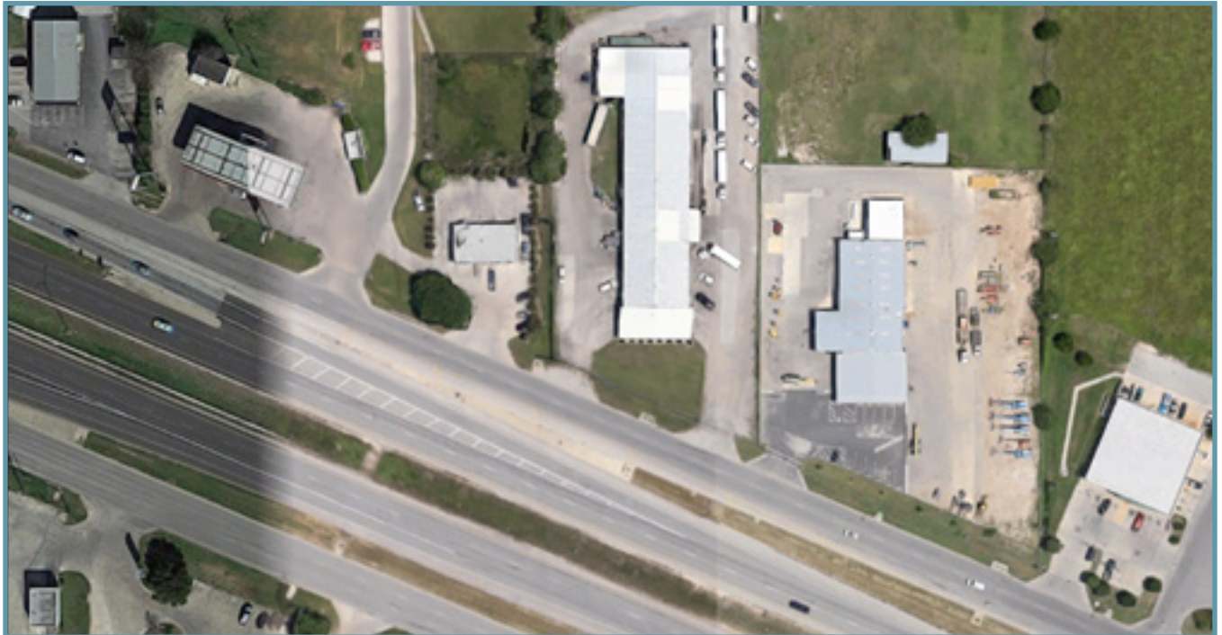
FIGURE 6.5, FREQUENT DRIVEWAY SPACING ON SH 71/21
