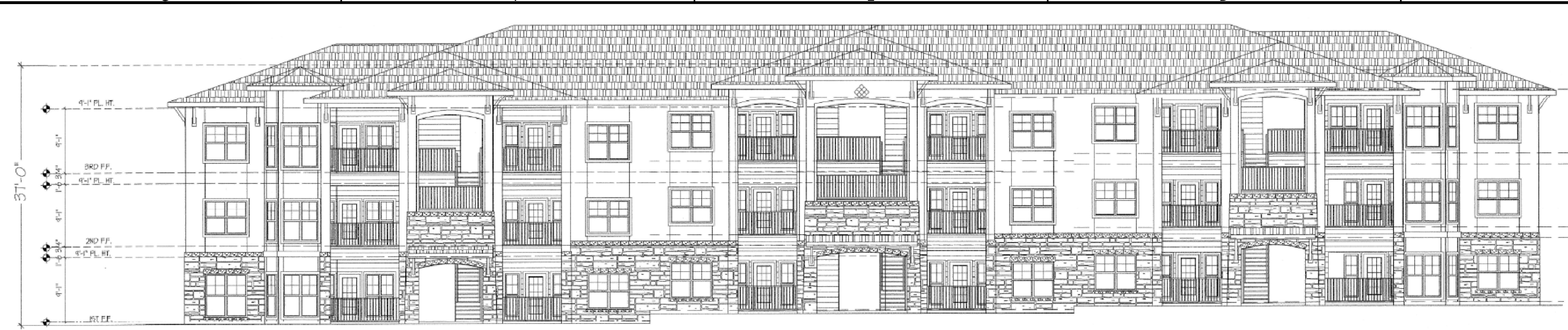
TYPICAL BUILDING FRONT ELEVATION NOTE: BUILDING HEIGHT IS MEASURED FROM AVERAGE SITE GRADE. 1"=16'
