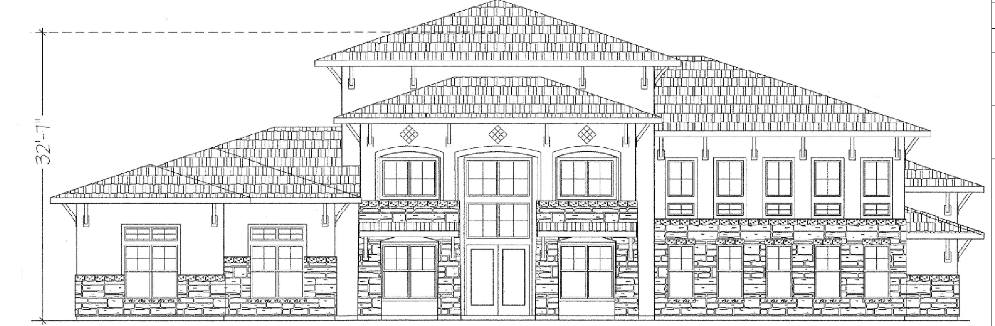
CLUBHOUSE FRONT ELEVATION NOTE: BUILDING HEIGHT IS MEASURED FROM AVERAGE SITE GRADE. 1"=16'
