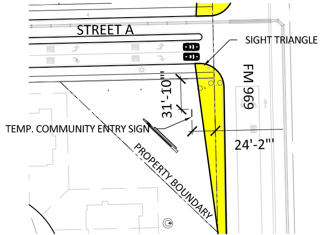
G-1 COMMUNITY ENTRY SIGN PROTOTYPICAL DETAIL PLAN Scale: 1" = 100' North
