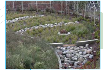
CONVEYANCE STORMWATER SLOWING THROUGH STONES + PLANTING
