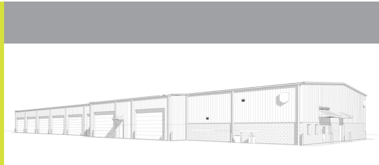
Pre-Engineered Metal Building, UPS Parcel Distribution Center
