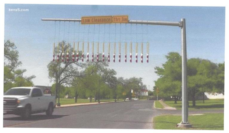
To stop future accidents under the Independence Avenue bridge, Kansas City is looking to install a warning curtain that would alert drivers of the low clearance. The city provided this photo as an example of what the new system could look like. Kansas City Communications Office
