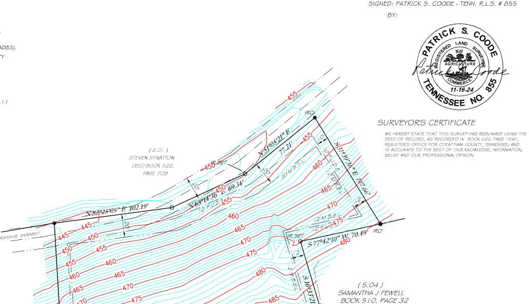
LOT 2 90,091.9 SQ, T. ± 2.07 AC ± 40 Цi POSSIBLE ABANDONED CIRCL SEPTIC TANK 35' (7'X7' CONCRETE WITH RAISED CIRCLE/LID) S 81°18'25" W 97.43' RVIEW S 03°02'41 LOT 1 12' SIDE 10,004.6 SQ. FT. ± SETBACK 0.23 AC ± **APPROXIMATE APPROXIMATE** 35' M.B.S.L. LOCATION R SEV LOCATION 4IN WATER LINE 80 GIN WATER LINE S 84°48'29" W 62.44' IR SE TN STATE PLANE COORDINATES (NAD83) \$ 84°48'29" W 134.78' IR SE BOYD STREET
