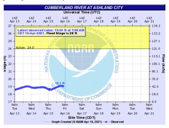
The River Gauge "0" reading is 367.04 ft (NAVD88). Thus a 20 ft. river gage reading calculates as elevation 387 ft. The summer pool elevation is around 385' at the Cheatham Dam. Nashville will be at a higher elevation, and Clarksville will be at a lower elevation. The 100-year flood level elevation is considered to be 402.3 ft (NAVD88) per the 2/26/21 FEMA flood map. The elevation of the top of the A.O. Smith flood abatement system is 409 ft.
