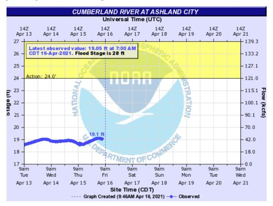
The River Gauge "0" reading is 367.04 ft (NAVD88). Thus a 20 ft. river gage reading calculates as elevation 387 ft. The summer pool elevation is around 385' at the Cheatham Dam. Nashville will be at a higher elevation, and Clarksville will be at a lower elevation. The 100-year flood level elevation is considered to be 402.3 ft (NAVD88) per the 2/26/21 FEMA flood map. The elevation of the top of the A.O. Smith flood abatement system is 409 ft.
