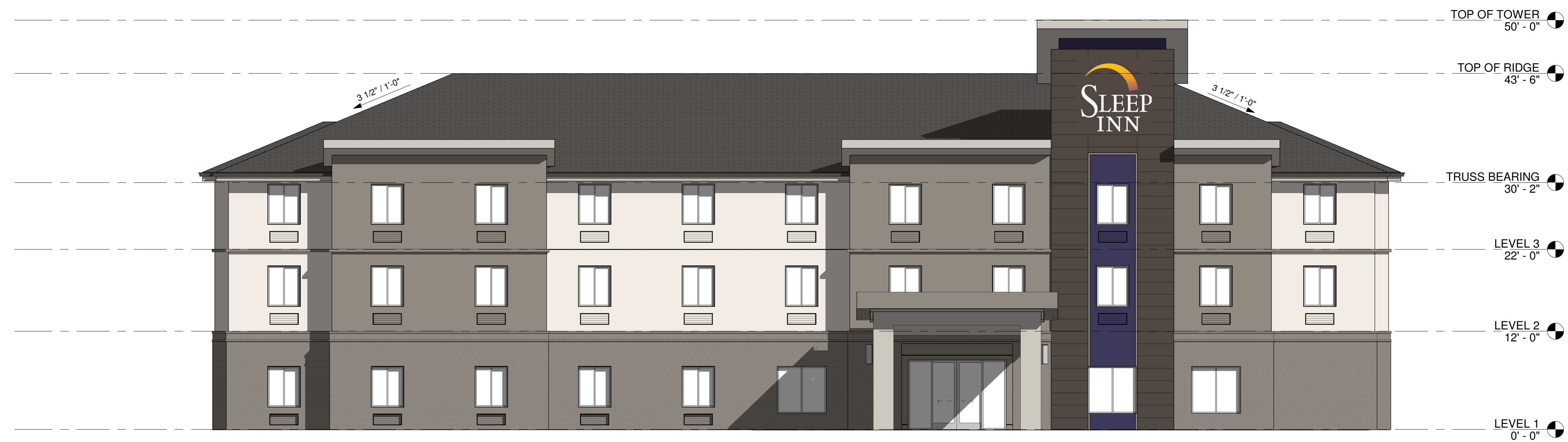
① front elevation 1/8" = 1'-0"
