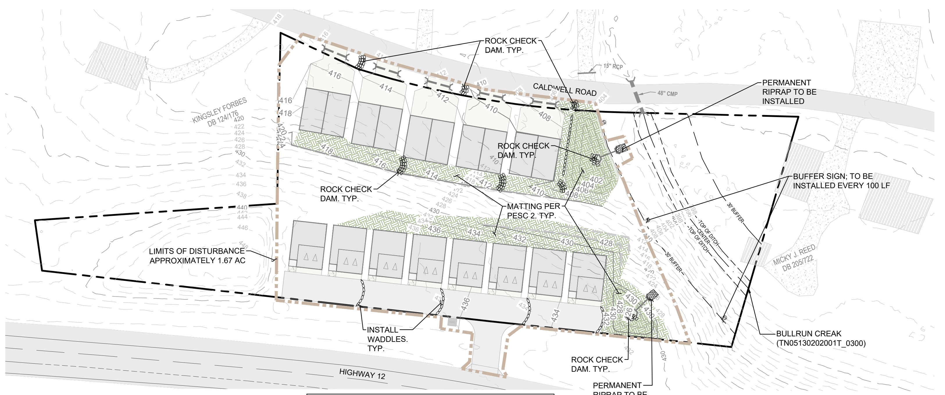
EROSION CONTROL - PHASE II
