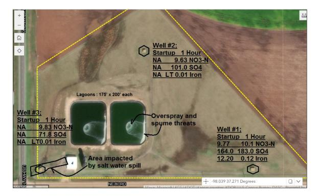
The lab data for these wells indicate Nitrates hover around the 10 mg/L value. The sulfates increase with pumping in Well #1 and are significantly higher than Wells #2 and #3. Again, this increase in Sulfates may impact plant efficiencies.
