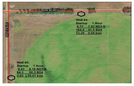
The increased Iron content in the startup samples indicates the presence of Iron bacteria and / or galvanic corrosion of the low carbon steel(LSC) casing. The corrosion process would provide Iron as a food source for the bacteria. In addition, the bacteria themselves will attack and feed off the LCS Ultimately, these processes can cause casing and some times screen failure in the well.
