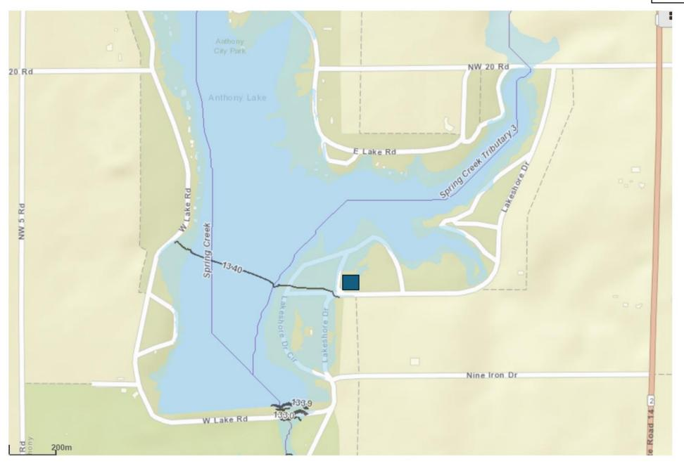
Lake Bathroom Review Map. Area in Blue denotes floodplain. Options to locate bathroom: 1. Construct in floodplain by adding stem walls to elevate lowest floor. 2. Locate outside of the floodplain.
