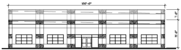
2 CONCRETE TILTWALL CONCEPTUAL ELEVATION SCALE: 3/32" = 1'-0"
