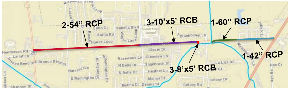
Figure 3. Proposed Storm Sewer System
