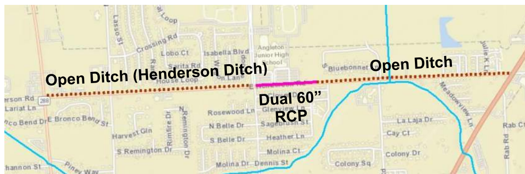
Figure 2. Existing Drainage System
