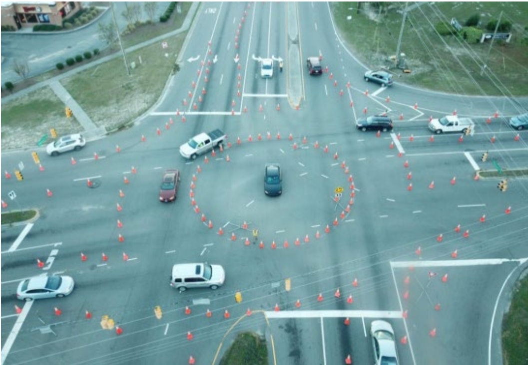
Figure 17. Example of a Temporary Roundabout Design
