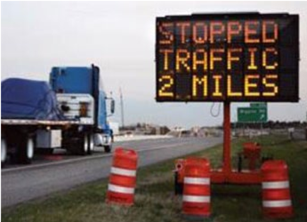
Figure 14. Example of a Portable Message Sign
