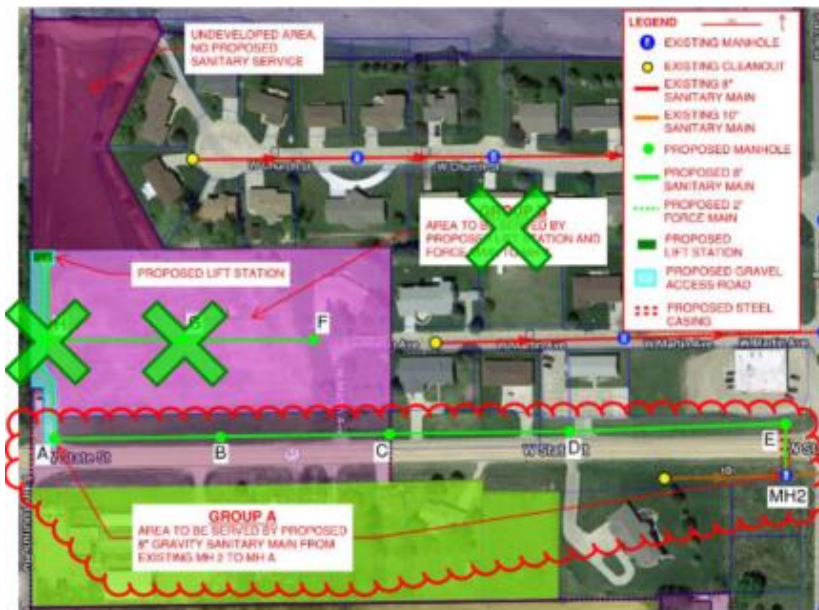
Figure 3: Sanitary Sewer Main for Annexation Area 1-B
